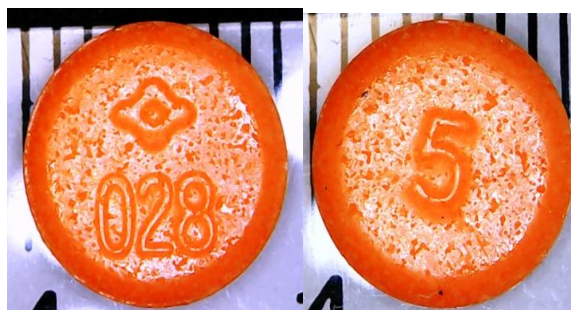
Figure 1: Physical observation on the imprint of Erimin-5 tablet.
