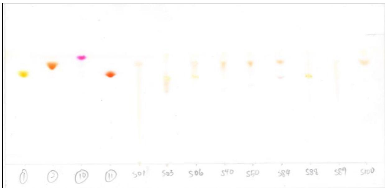
Figure 9: TLC output of illicit Erimin-5 samples in comparison to the dye standards using solvent system consisting of isopropanol: ammonia: water (7:2:1 v/v/v).
